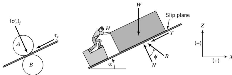
**FIGURE 10.11** Simulation of failure in dense sand.
