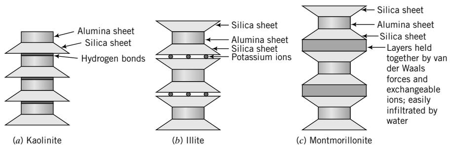
**FIGURE 2.7** Structure of kaolinite, illite, and montmorillonite.
