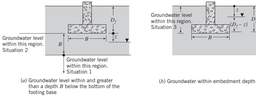
**FIGURE 12.12** Groundwater effects below base of footing.
