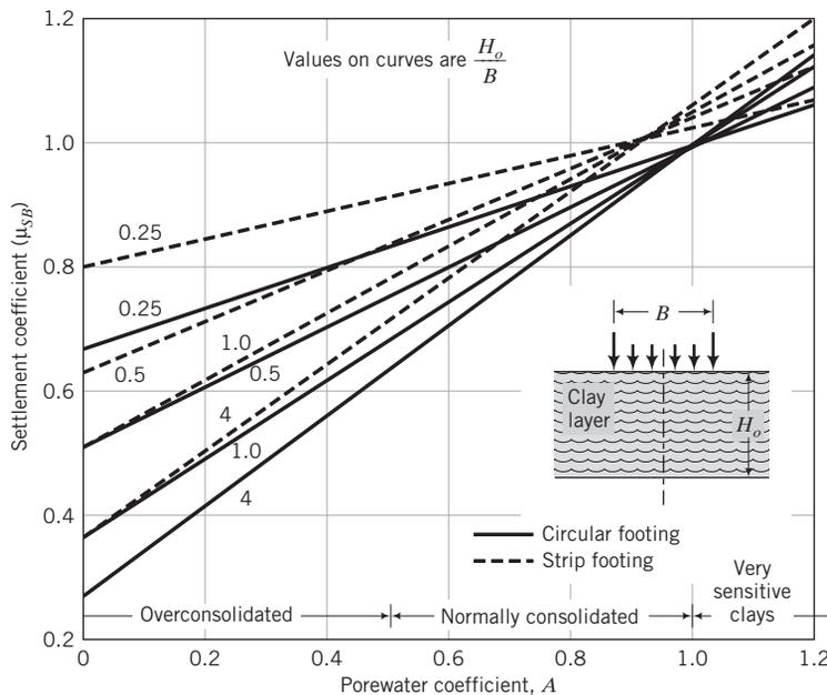
**FIGURE 12.17** Values of  $\mu_{SB}$  for circular and strip footings. (Redrawn from Scott, 1963.)
