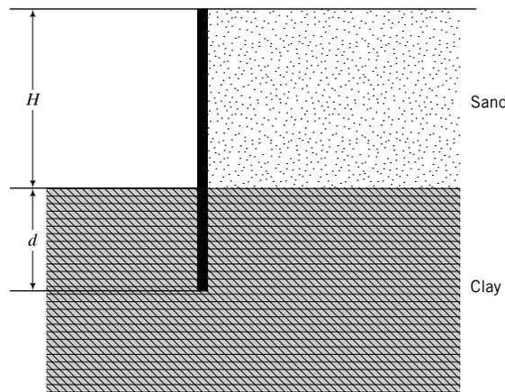
**FIGURE 15.20** Sheet pile wall penetrating different soils.
