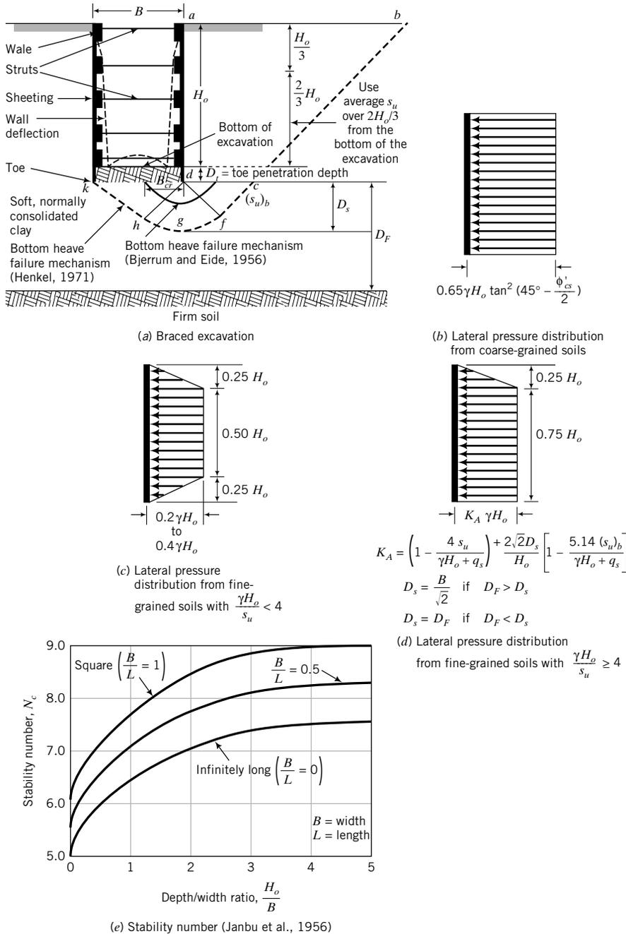
FIGURE 15.26 Braced excavations.
