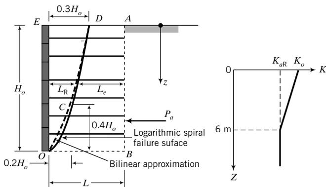
**FIGURE 15.31** Coherent gravity method.
