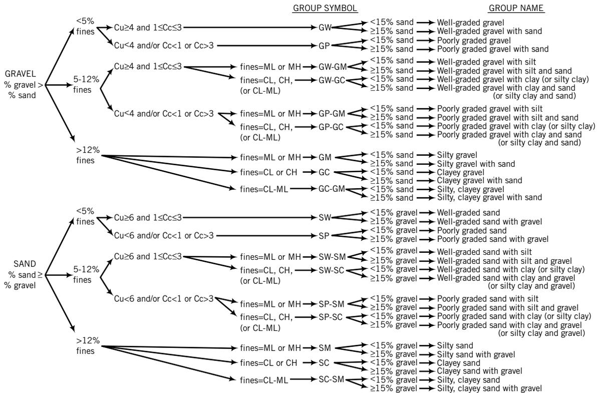
**FIGURE 4.10a** Flowchart for classifying coarse-grained soils more than 50% retained on No. 200 sieve. (Source: Reprinted with permission from ASTM D 2487-10 Standard Practice for Classification of Soils for Engineering Purposes, copyright ASTM International, 100 Barr Harbor Drive, West Conshohocken, PA 19428.)
