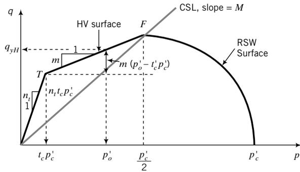
**FIGURE 11.31** Hvorslev's limiting stress surface within CSM.
