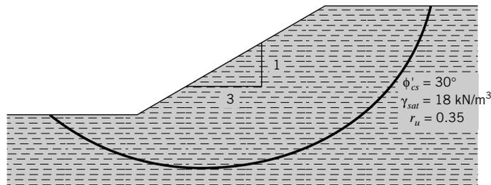
**FIGURE E16.7****Strategy** Use the Bishop and Morgenstern (1960) charts and equations. Follow the procedures in Section 16.11. Since you are given  $r_u$ , you only need to do Steps 4 and 5.**Solution 16.7****Step 1:** Determine  $m$  and  $n$ .From Figure 16.13,  $m = 1.73$  and  $n = 1.92$  for a slope of 3:1 and  $\phi'_{cs} = 30^\circ$ .**Step 2:** Calculate FS.
