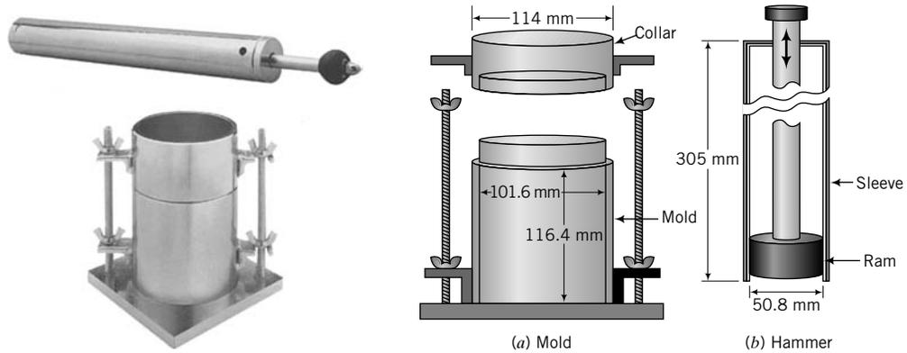
**FIGURE 5.3** Compaction apparatus. (Photo courtesy of Geotest.)
