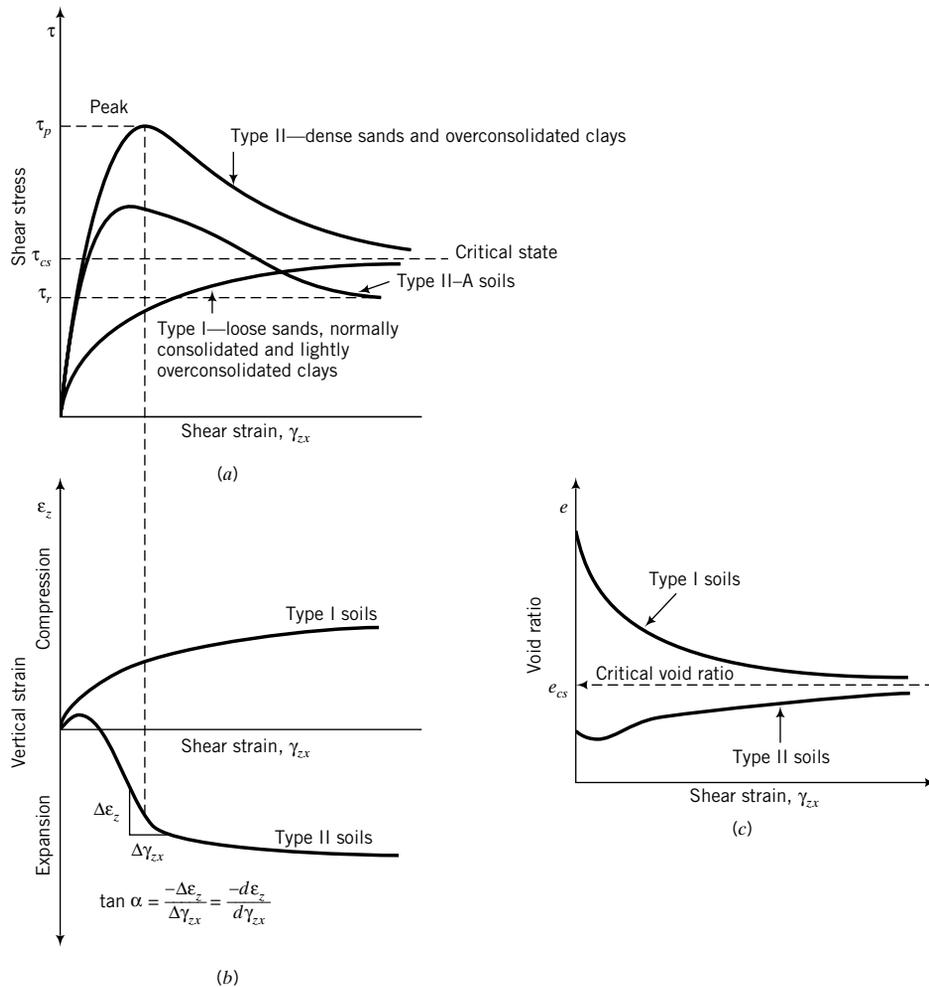
**FIGURE 10.3** Response of soils to shearing.
