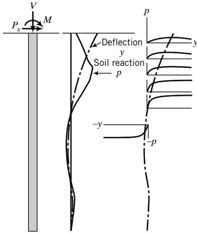
**FIGURE 13.23** Pile-soil response to lateral loads and moments.
