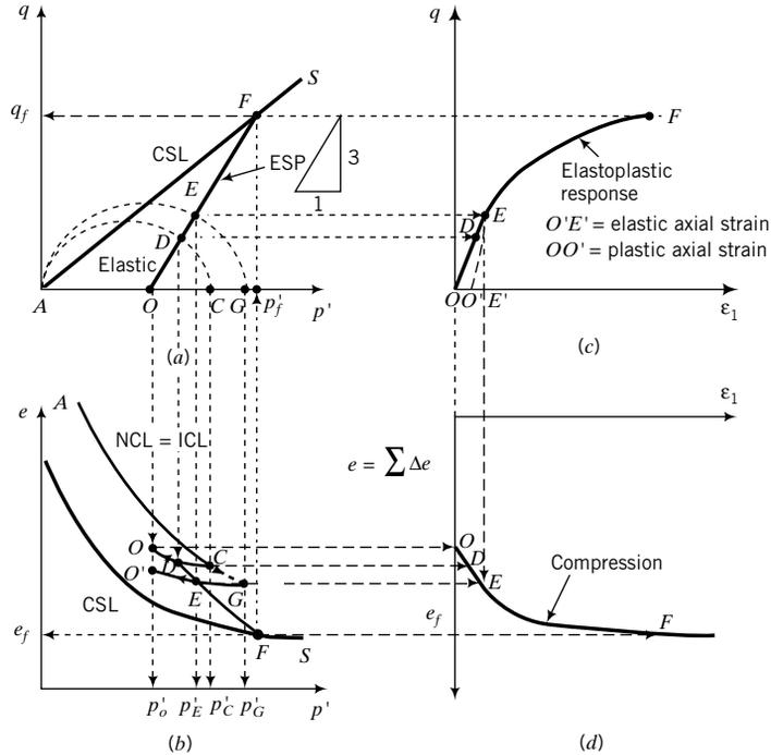
**FIGURE 11.4** Illustrative predicted results from a triaxial CD test on a lightly overconsolidated soil ( $1 < R_o \leq 2$ ) using CSM.
