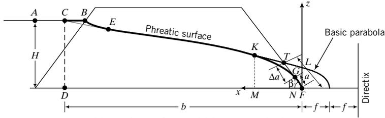
**FIGURE 14.9** Phreatic surface within an earth dam.
