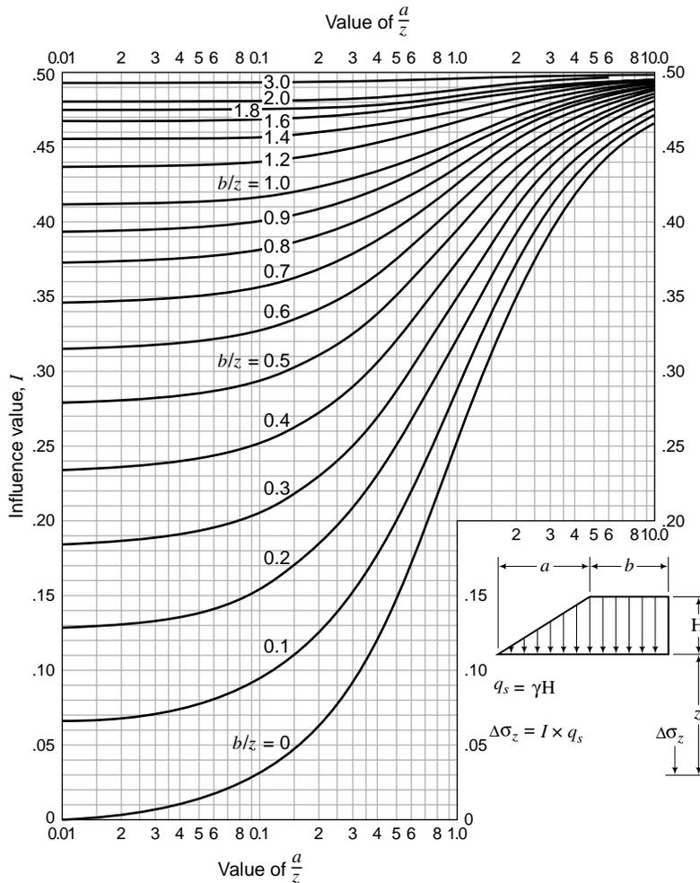
**FIGURE 7.27** Vertical stress increase due to an embankment.
