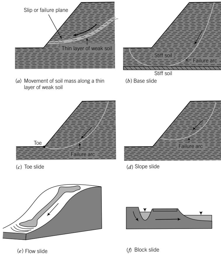
**FIGURE 16.2** Some common types of slope failure.
