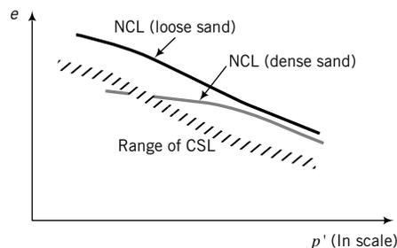
**FIGURE 11.10** Illustrative volumetric responses of coarse-grained soils.
