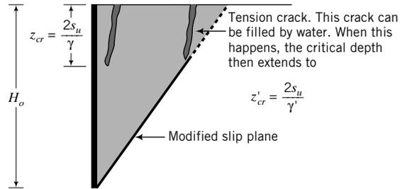
**FIGURE 15.12** Tension cracks behind a retaining wall.
