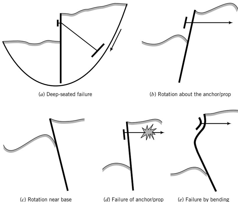
**FIGURE 15.16** Failure modes for flexible retaining walls.
