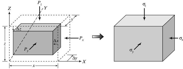
FIGURE 7.2 Stresses and displacements due to applied loads.
