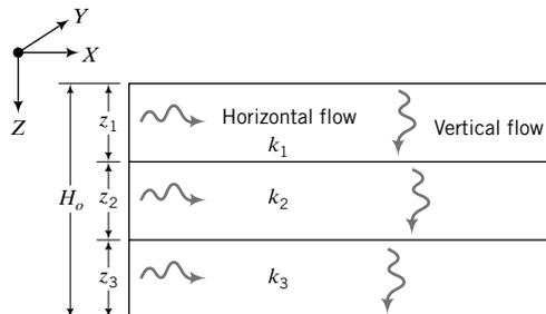
FIGURE 6.6 Flow through stratified layers.
