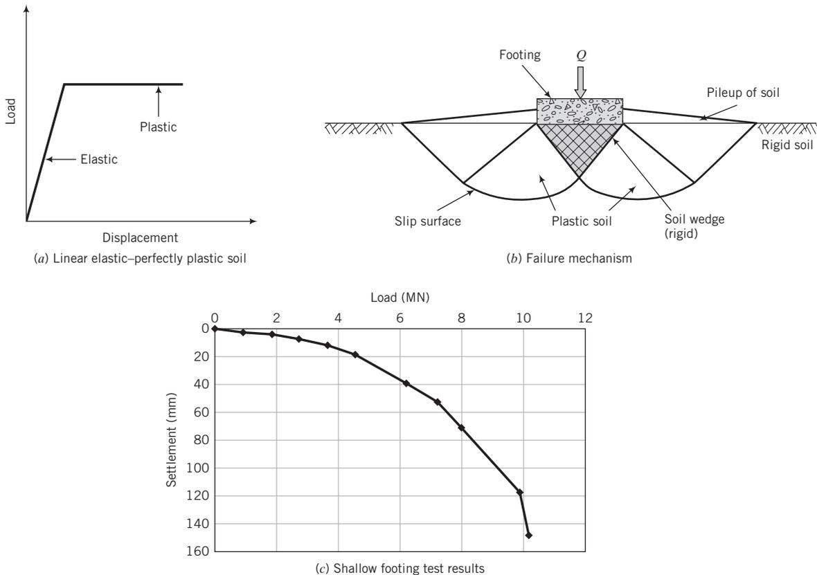
**FIGURE 12.3** (a) Load–displacement response of an elastic–perfectly plastic material. (b) Indentation of soil wedge into a soil (no slip at the wedge faces and at the footing–soil interface; slip along the footing thickness). (c) Field test results of a 3-m-square footing on a sand. (Data from Briaud and Gibbens, 1994.)
