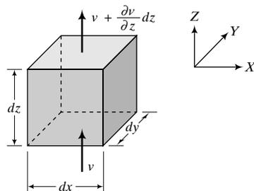
FIGURE 9.6 One-dimensional flow through a two-dimensional soil element.
