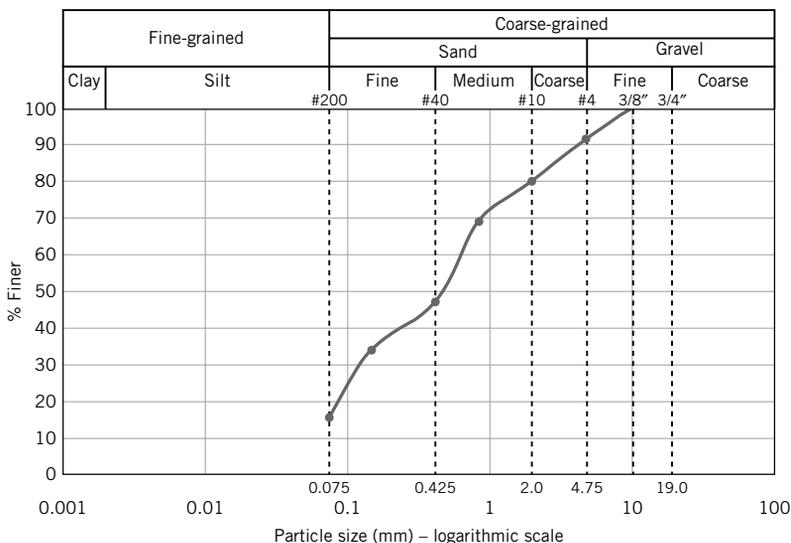
**FIGURE E2.1** Grading curve.
