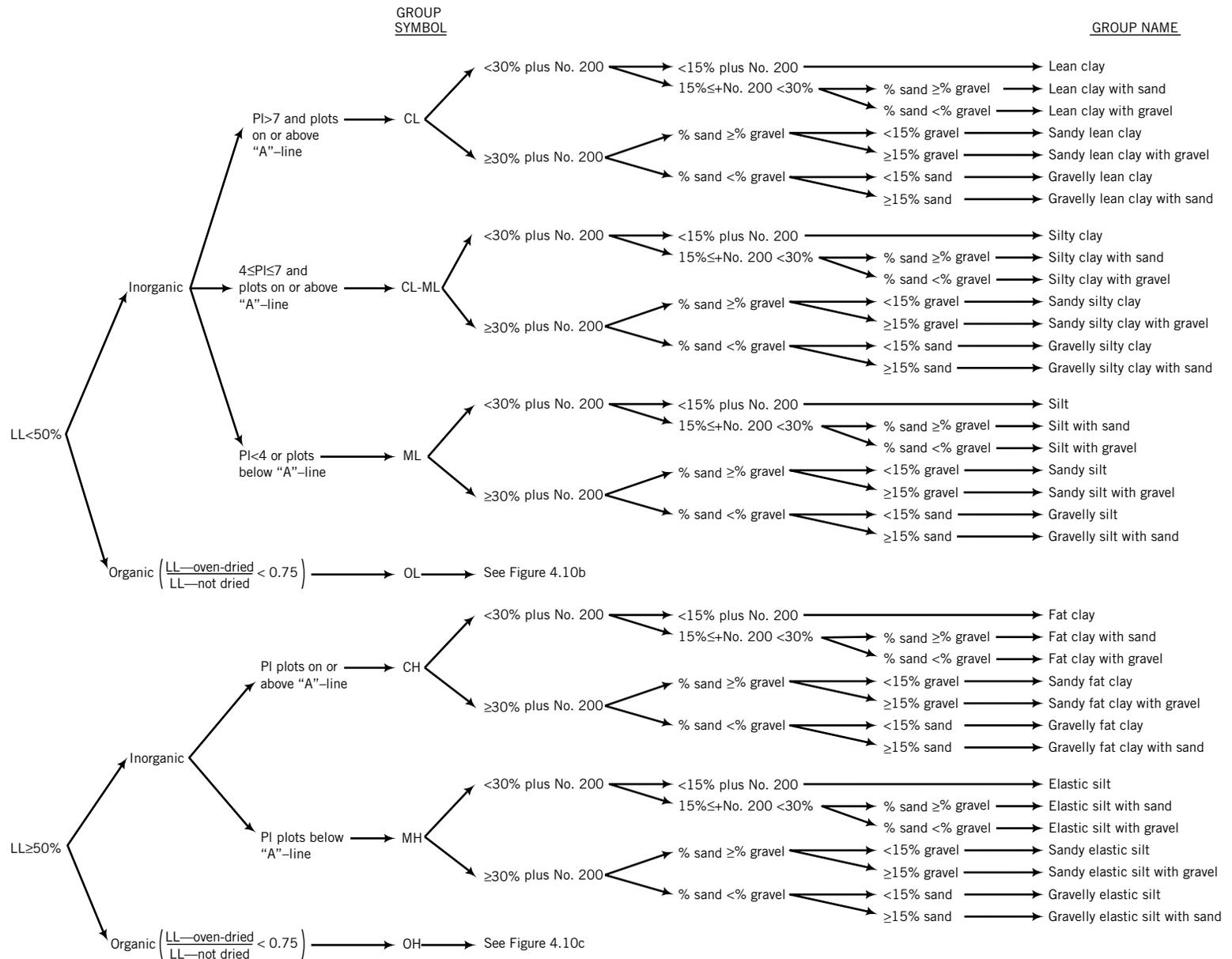
**FIGURE 4.10b** Flowchart for classifying inorganic fine-grained soils (50% or more fines). (Source: Reprinted with permission from ASTM D 2487-10 Standard Practice for Classification of Soils for Engineering Purposes, copyright ASTM International, 100 Barr Harbor Drive, West Conshohocken, PA 19428.)
