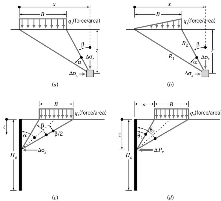
**FIGURE 7.22** Strip load imposing (a) a uniform surface stress and (b) a linear varying surface stress. (c) Strip load imposing a uniform surface stress near a retaining wall and (d) lateral force on a retaining wall from a strip load imposing a uniform surface stress.
