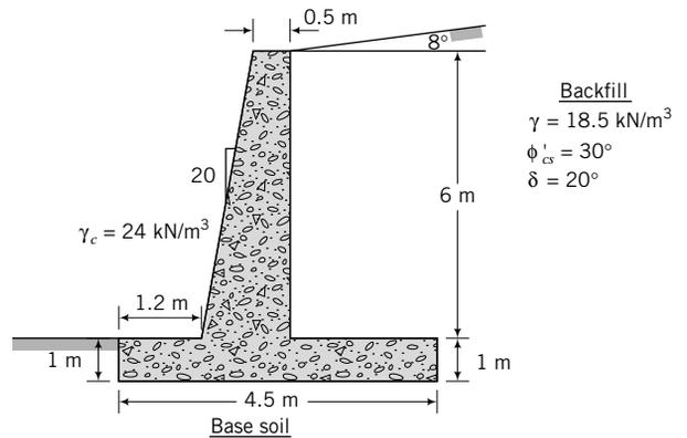
Clay:  $\gamma = 19 \text{ kN/m}^3$ ,  $\phi'_p = 30^\circ$ ,  $\phi'_b = 20^\circ$ ,  $s_u = 94 \text{ kPa}$
