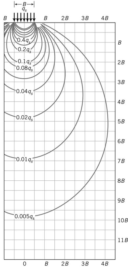
**FIGURE 7.23** Vertical stress contour below a square foundation.
