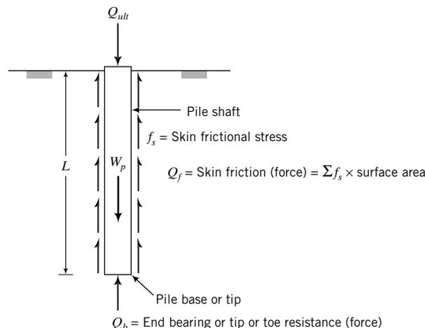
**FIGURE 13.9** Pile shaft and end bearing resistance.
